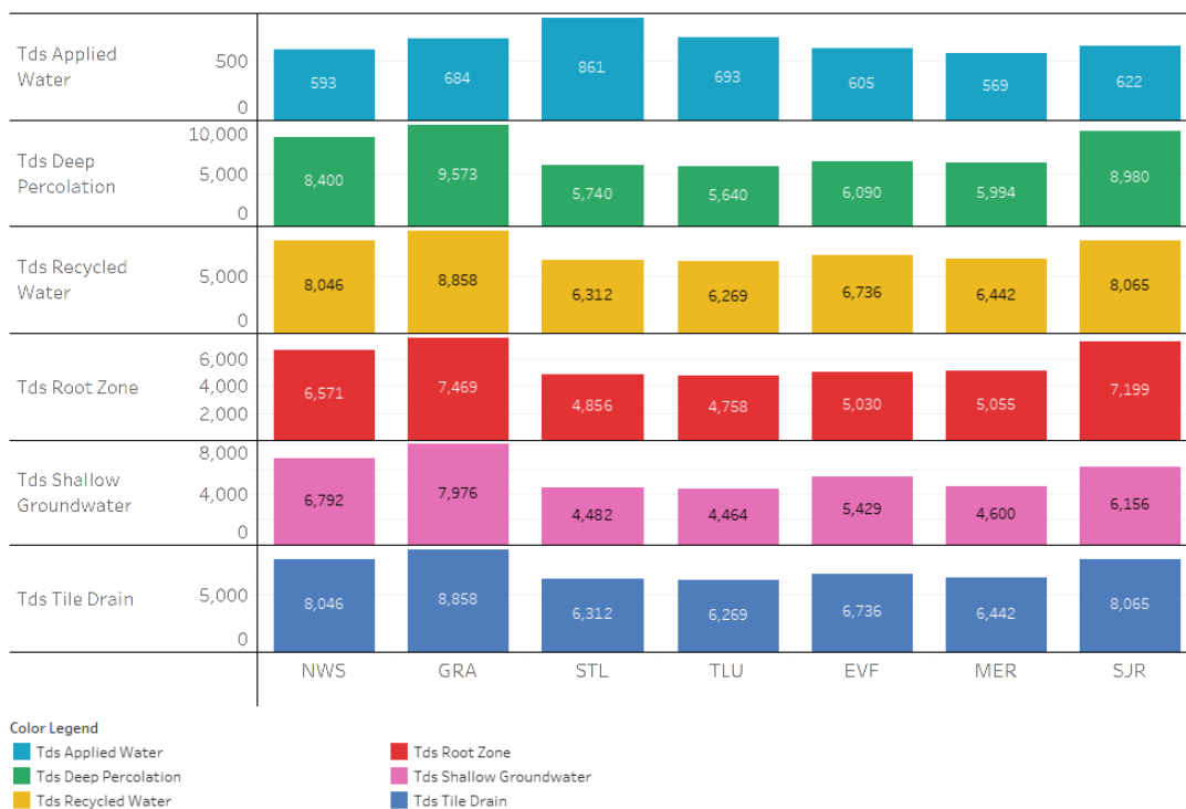
Figure 10. Model-produced concentration of salinity as total dissolved solids (TDS) for water sources within the model including all applied water, deep percolation, recycled water, root zone, shallow groundwater, and tile drain (drainage water).
